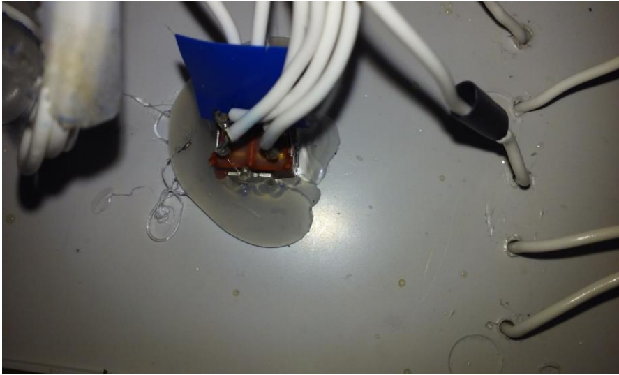
7 Mode switch wired and glued.
