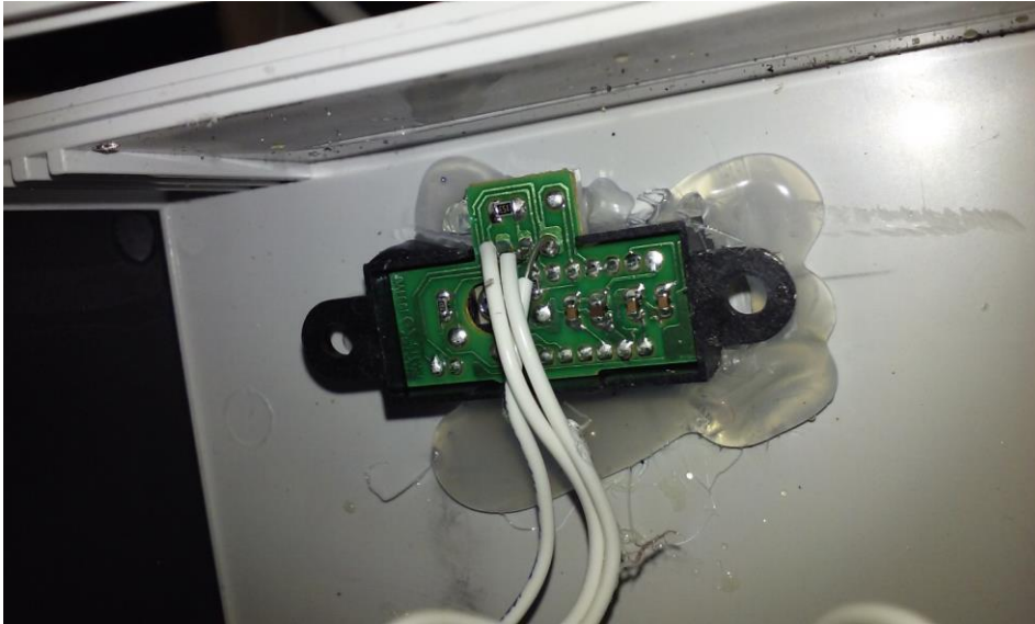
9 IR sensor glued and wired
