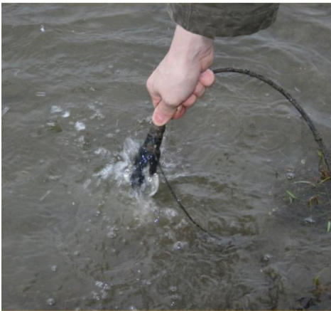
3. Initial cleaning to remove mud and debris from the connector face can be done by rinsing in water. A hose, bucket of water, stream or muddy puddle will do.
