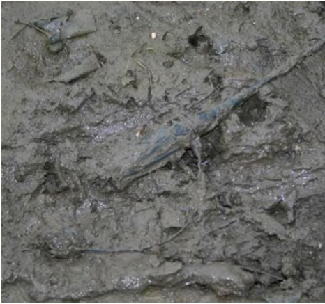
1. Plug connector immersed in mud. The connector is fully sealed even without the dust cap fitted.
