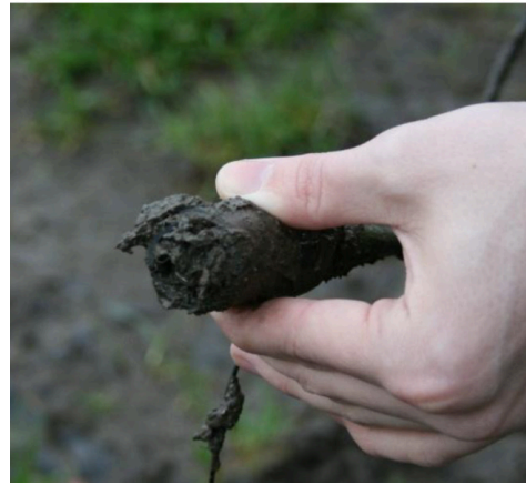
2. The mud will not cause damage to the insert. A physical contact connector would almost certainly already be destroyed in this state.
