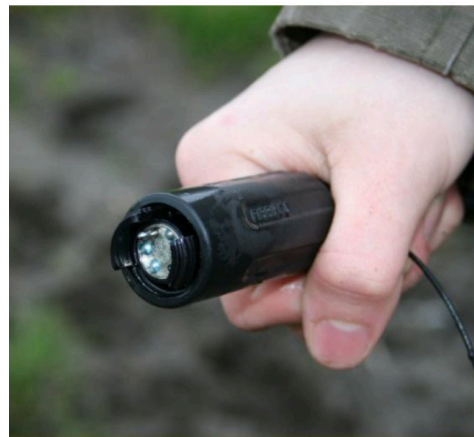
4. Connector end-face is clean after rinsing.
