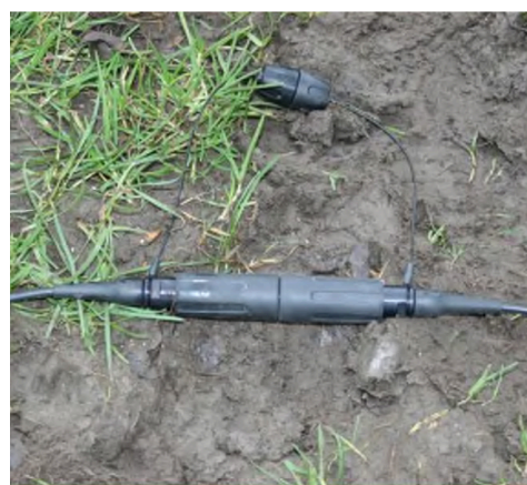
6. Connectors plugged and ready for service.
