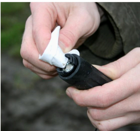
5. The insert face is dried and wiped clean. Ideally a clean cloth or tissue is used but if these are not available the bottom of your coat will suffice. No damage to the insert surfaces or lenses will occur.
