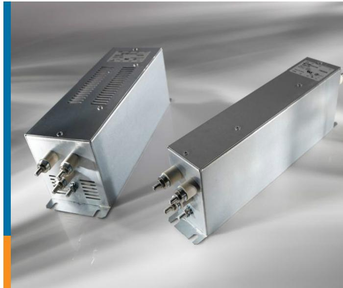
TE Connectivity (TE) introduces the new BCF series power line filters with threaded stud terminals. Previously available in terminal block terminations only, the new low-weight BCF series is a 3-phase Delta EMI filter with threaded terminals for easy termination to cables with ring terminals. These new filters are used to reduce noise emissions typically associated with variable speed motors used in process automation equipment, elevators and alternative energy applications.
