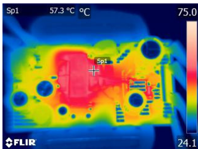
Figure 20 – Transformer Side. 265 VAC, Full Load.
