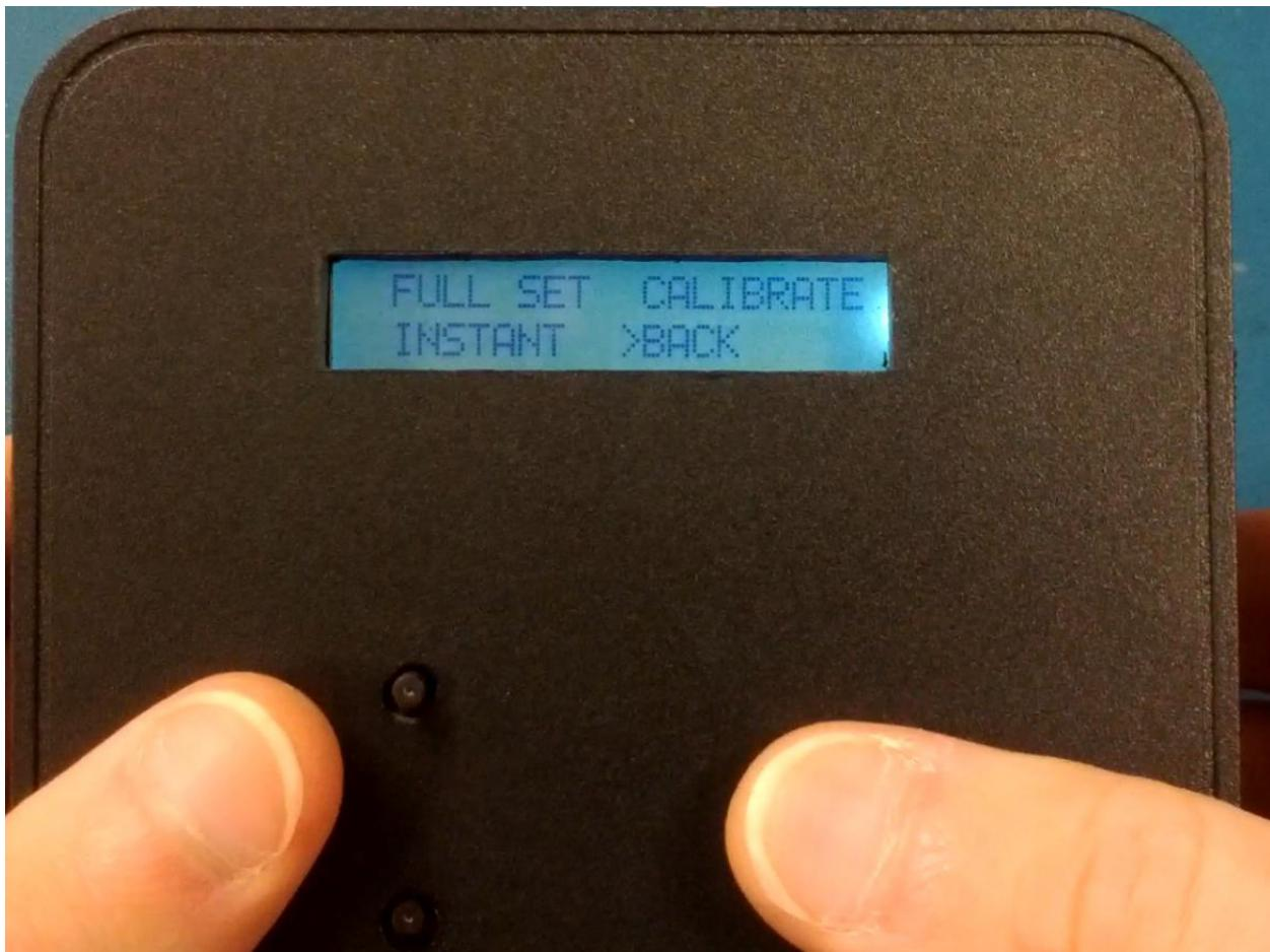
Next, navigate to RECALL, hit select, then navigate to the memory slot you want to look at and press select again. Then advances to the most complicated display on this pyrometer device:
