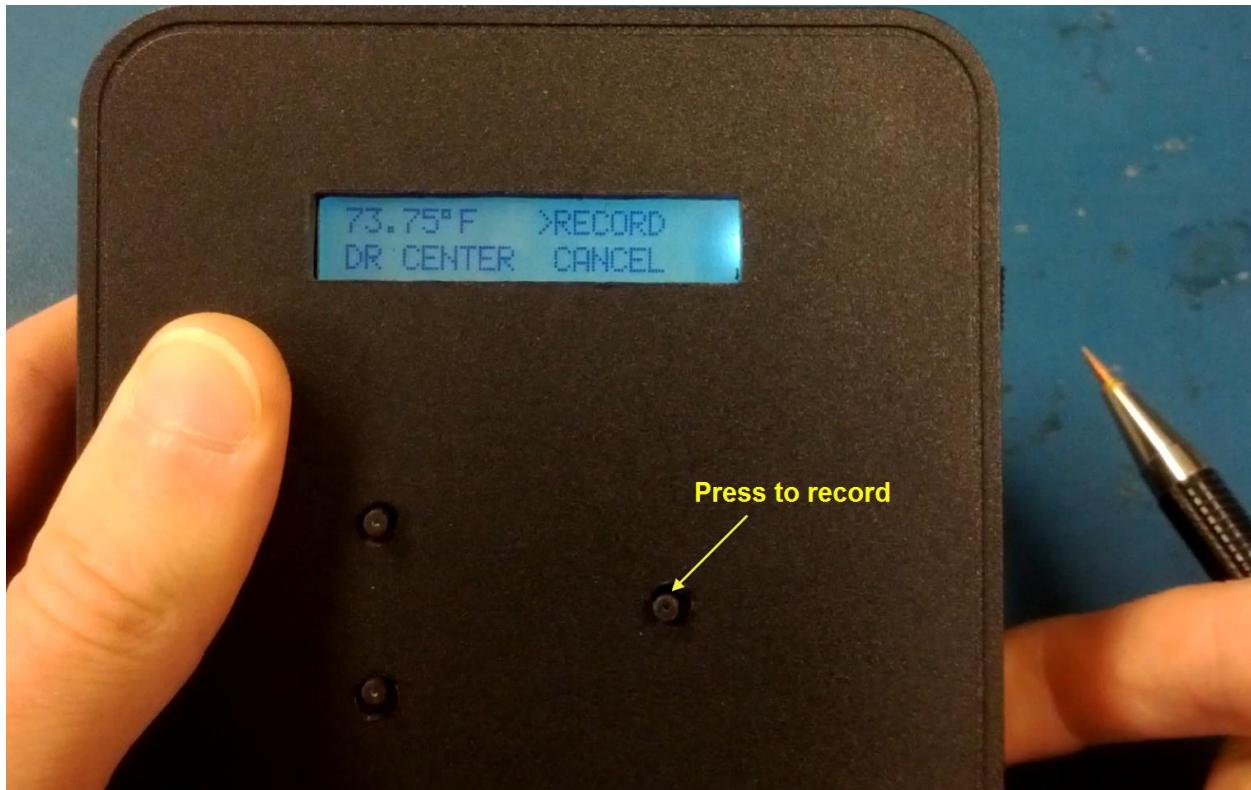
When you press the right button while on >RECORD, the pyrometer MCU immediately advances the menu to driver side (D), rear tire (R), CENTER probe position (on the tire.) So now you put the probe on the center of the same tire, wait for the temperature to stabilize, then hit record again. The menu then advances to DR OUTER.
