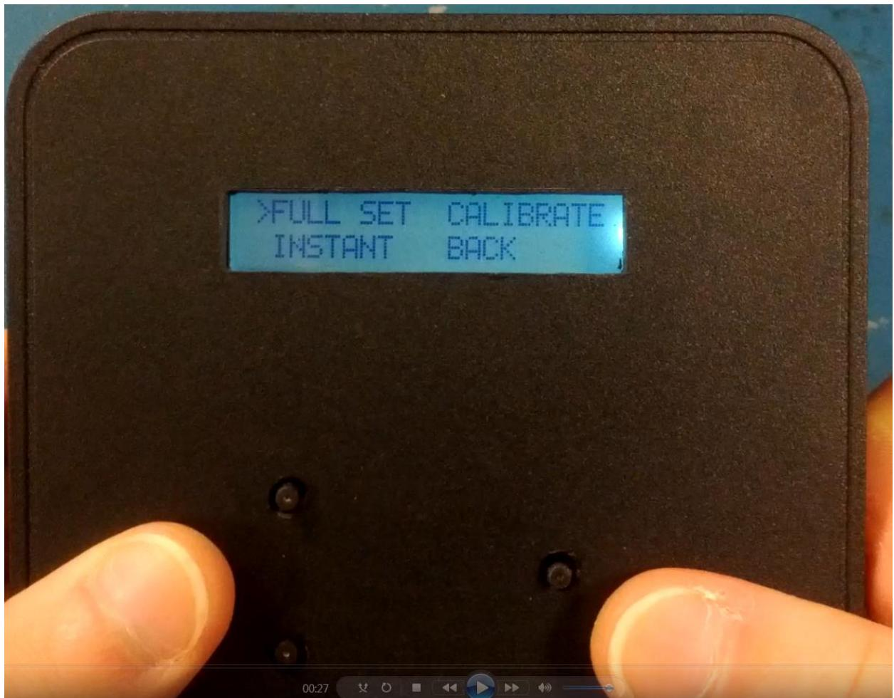
FULL SET means that you will be probing all four tires and taking three temperature measurements per tire for 12 measurements total. Or you can go into the instantaneous (INSTANT) mode which will show you a live temperature feed. So I navigate to INSTANT using the left bottom button. Since I'm indoors it looks like this:
