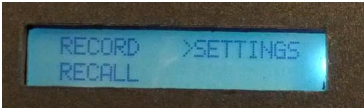
If you go into the SETTINGS menu and then into MEMORY, it allows you to export your data to .CSV (comma separated) via the serial port at the top of the box:
