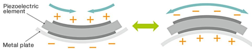
There are two types of piezoelectric elements; single-plate and multilayer. Since the PiezoHapt™ Actuator has multilayer type, it can generate a larger displacement than that of single-plate element of the same thickness. Therefore, while high voltage is required for the piezoelectric-type haptic technology in general, TDK’s PiezoHapt™ Actuator can transmit a vibration sensation to the skin even at a low voltage of 24V.
