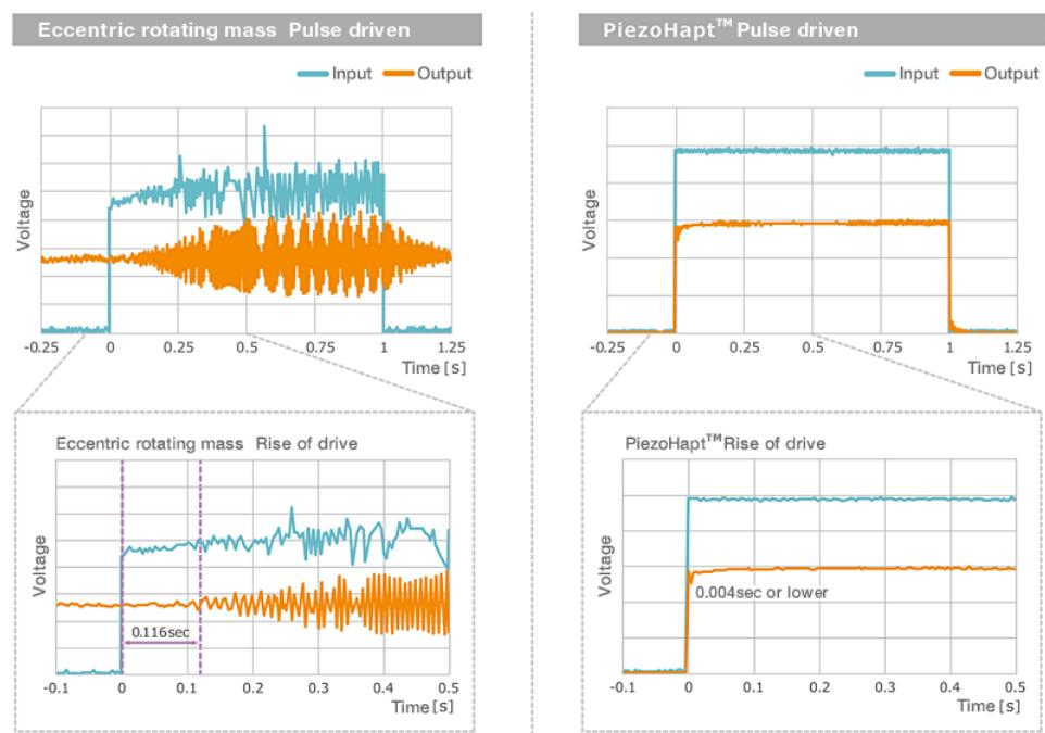
As shown in the graph below, with the PiezoHapt™ Actuator which can change the amplitude with drive voltage, it is possible to express various, delicately controlled vibration patterns.
