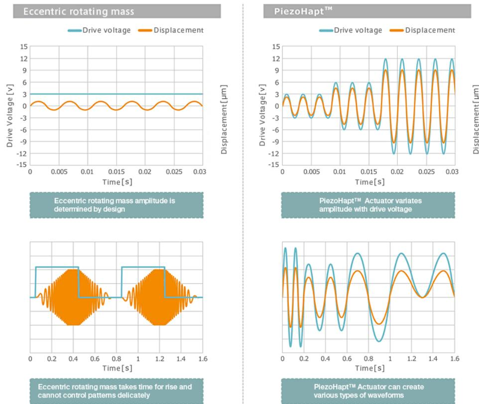
With this quick response and free amplitude control, the PiezoHapt™ Actuator can form the feedback base of vibration to the fingertip in various patterns and displacements, which expands the possibility of haptic feedback utilization.
