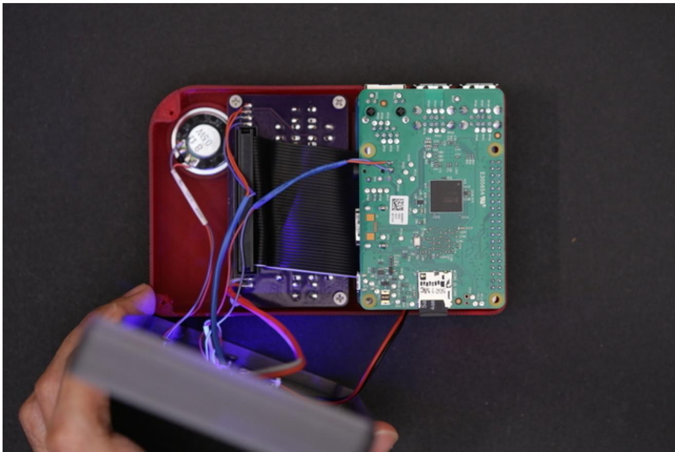
The best location for the battery I've found is directly tucked inbetween the Raspberry Pi and the PiTFT display.
