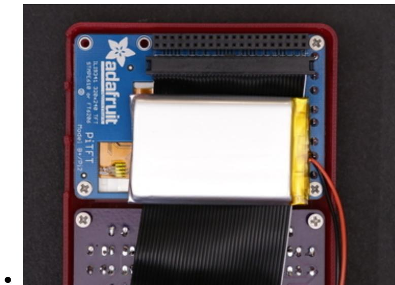
lipo battery. A good spot for it is right behind the PiTFT display. To keep it in place, we can use a piece of gaffers tape. Try to keep it up closely against PiCable. Position it like in the photo, closer to the right side to avoid intersecting with some of the components from the Pi.
