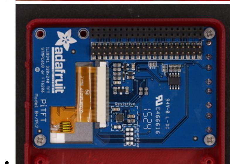
holes with the standoffs. Then, insert #4-40 3/8 sized machine screws into each mounting hole and fasten them into place. Be careful not to apply excess force, and fasten slowly.
