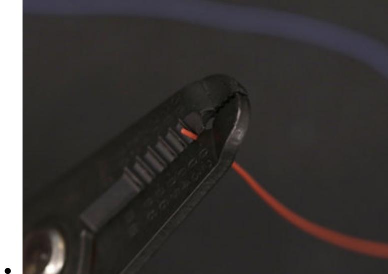
Use a pair of wire strippers to remove about 4mm of insulation from the tips of each wire. To keep the tips of wires from fraying, use the tip of the soldering iron to apply solder. You can bundle the tips of wires together and use a pair of helping third hands to tin the tips at the same time.
