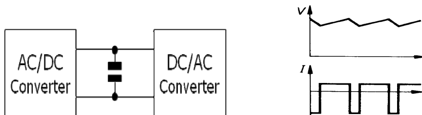
Figure 7: Snubber circuit scheme & typical waveforms on DC-Link caps
