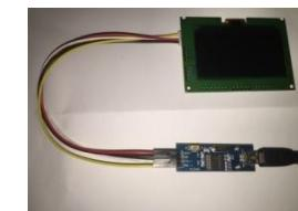
**Step 4 : Connect cable to OLED or Dot matrix LED Display module**
