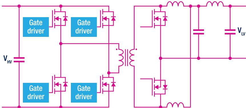
Primary: Super-junction MOSFETs with fast switching diode or IGBTs with copacked diode, in through-hole or SMD packages.
