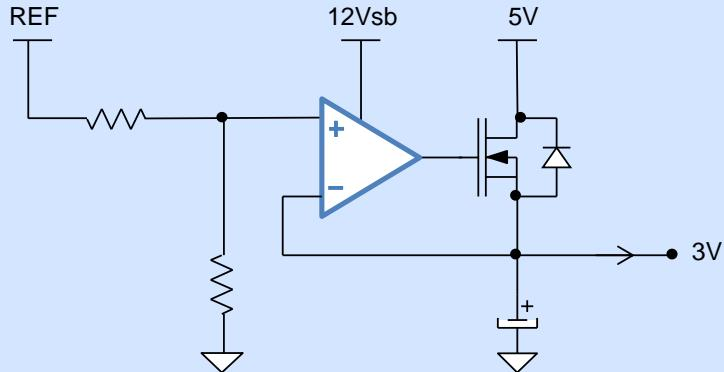
The op amp is driving the gate of a power Mosfet used as a linear regulator.
