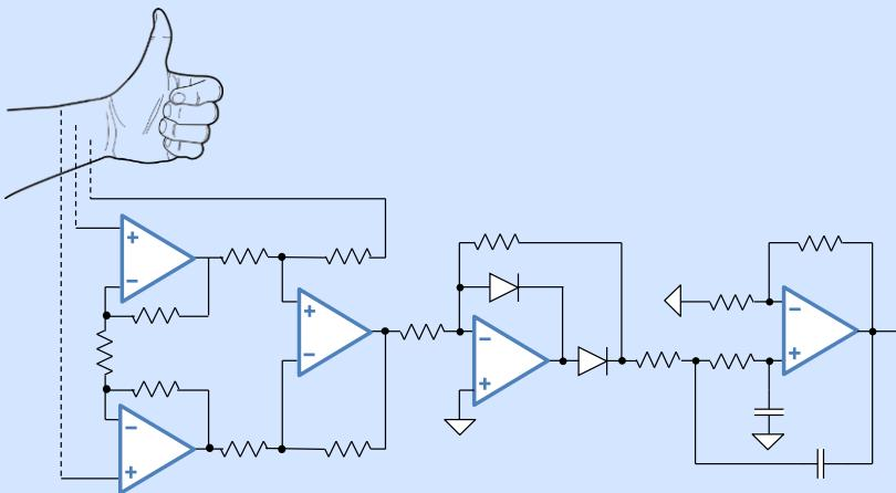
Surface EMG signals are amplified by op amp in instrumentation configuration, then rectified and filtered to provide feedback to digital system.
