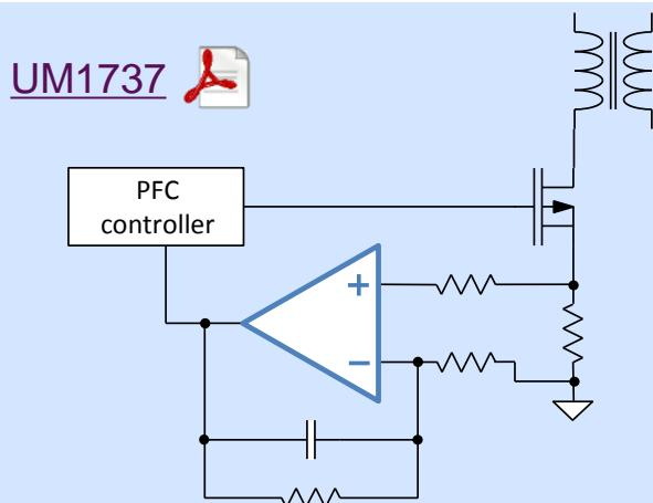
The current of the power Mosfet is measured by a shunt resistor. The resulting voltage drop is amplified and filtered by the op amp and feedback to the controller.
