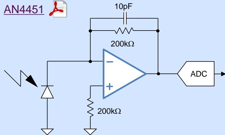
The photodiode generates a reverse current proportional to the amount of light. This current is converted into voltage and amplified by op amp.
