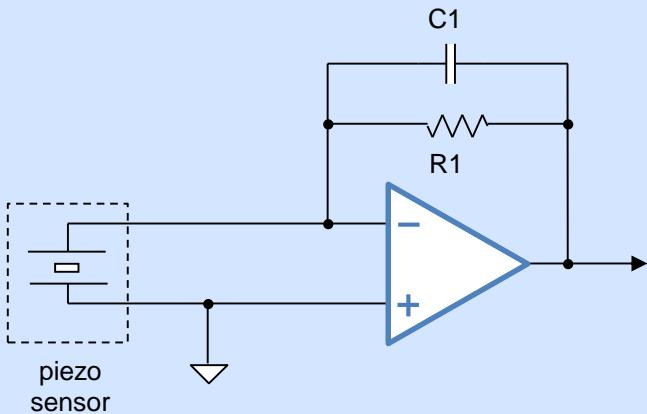
The shock is detected by a piezo sensor, creating an electrical charge at its electrodes. The charge is converted into voltage and amplified by op amp.
