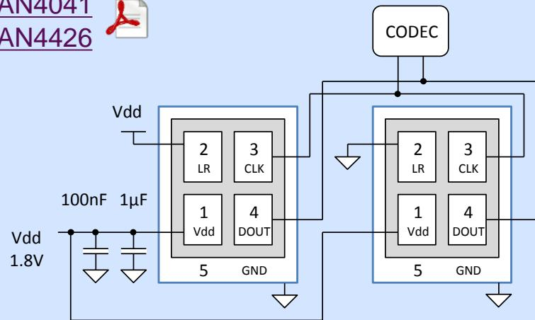
An array of microphones are working together to provide omnidirectional sound recording.
