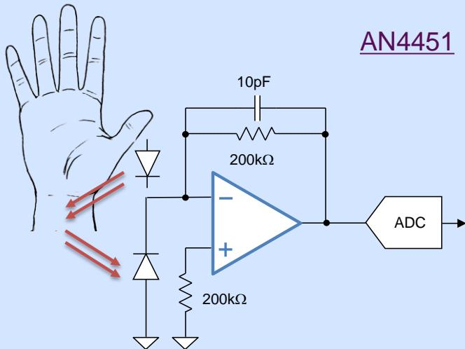
The LED emits light into the skin of the user. The reflected light - synchronized with heart pulses - is measured by op amp in trans impedance configuration.
