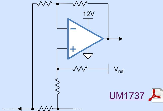
The output current of the power supply is measured on low-side by a shunt resistor. The resulting voltage drop is amplified by op amp.
