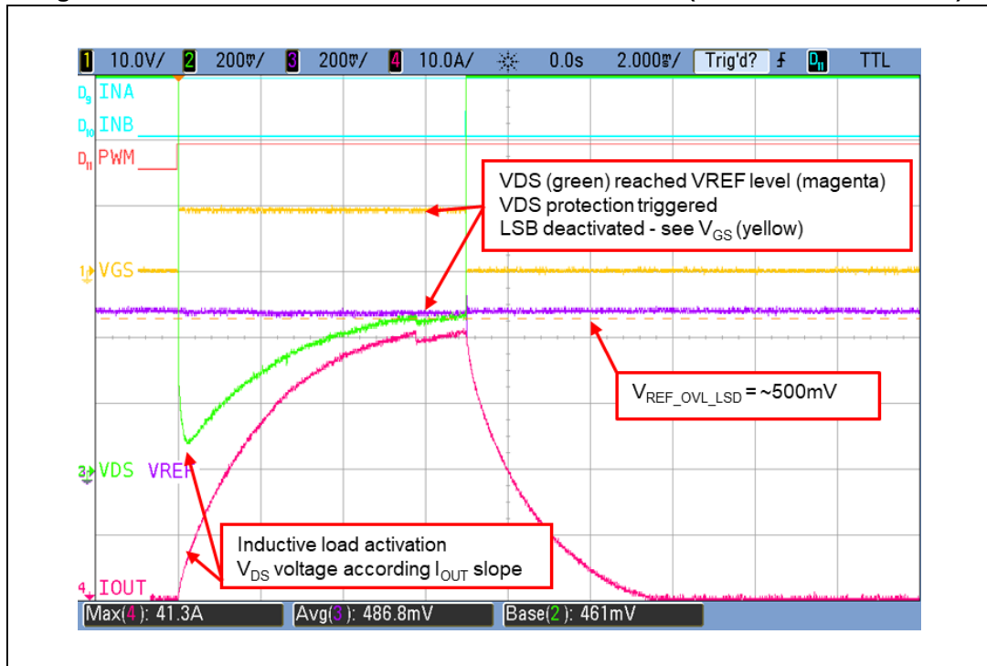
Figure 21. Load activation with too low VREF_OVL_LSD (RREF_OVL_LSD = 10k)
