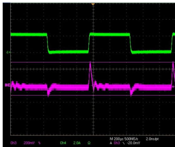
Fig. 5 - Green = Load Current, Purple = V_{out} Ripple Voltage, +240 mV, -80 mV
