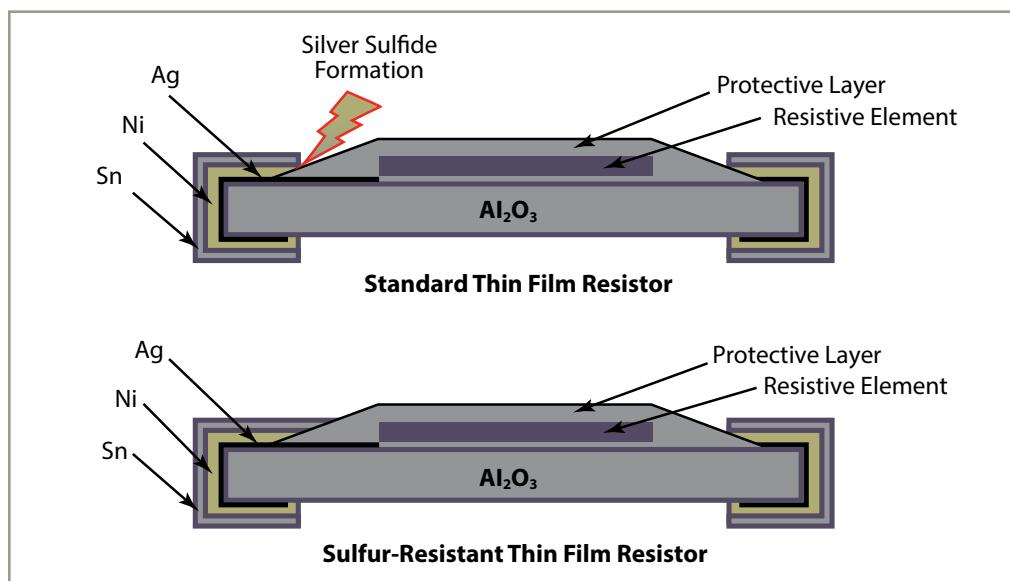
Figure 2. | Cross Section Showing Standard Thin Film Resistors vs. Sulfur-Resistant Thin Film Resistors
