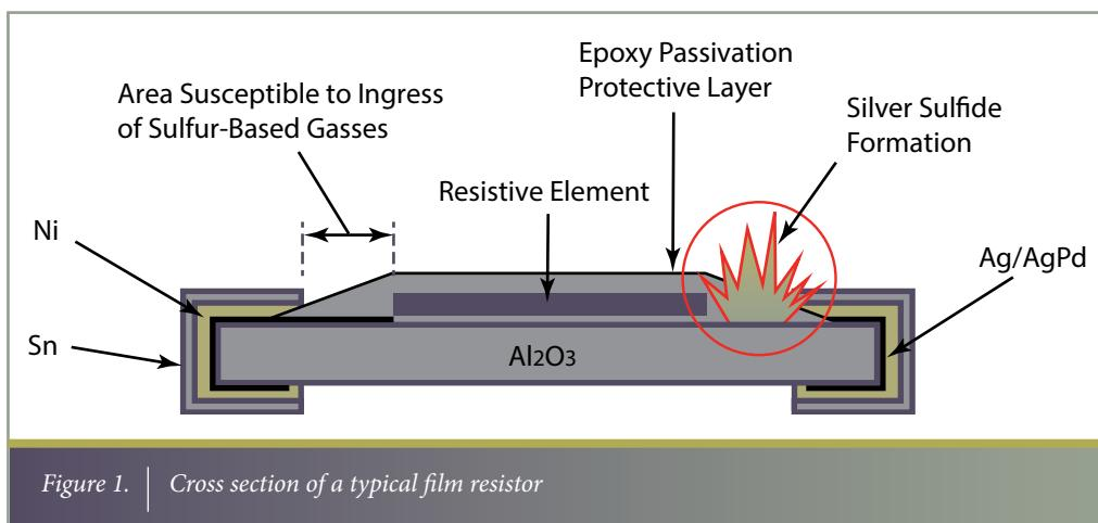
Figure 1. | Cross section of a typical film resistor
