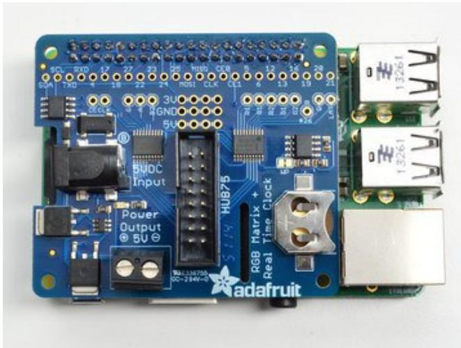
Shut down your Pi and remove power. Plug the HAT or Bonnet on so all the 2x20 pins go into the GPIO header.
