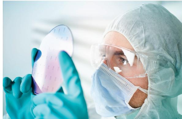
Storage time for wafers in sealed condition shall not exceed 6 months (storage ambient conditions:  $T_A = 15\ldots30^\circ\text{C}$ ; relative humidity: < 60 %).
