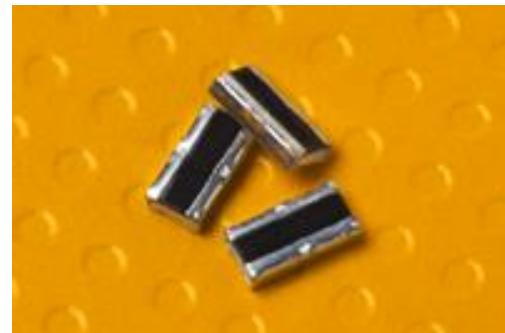
The WU73 chip resistor features wide side electrodes which provide better heat dissipation and smaller size compared to other standard chip resistors. This wide terminal resistor is designed for high accuracy and current detection, making it ideal for automotive, telecommunication and consumer electronic markets, in applications such as power supplies, DC to DC conversion and AC adaptors, Automotive ECU and motor circuits.
