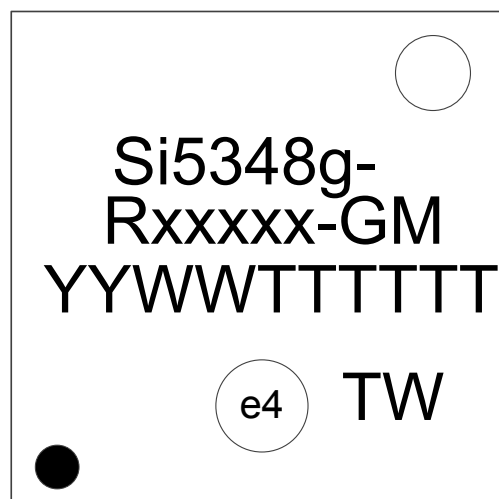
Figure 13.1. Si5348 Top Marking
