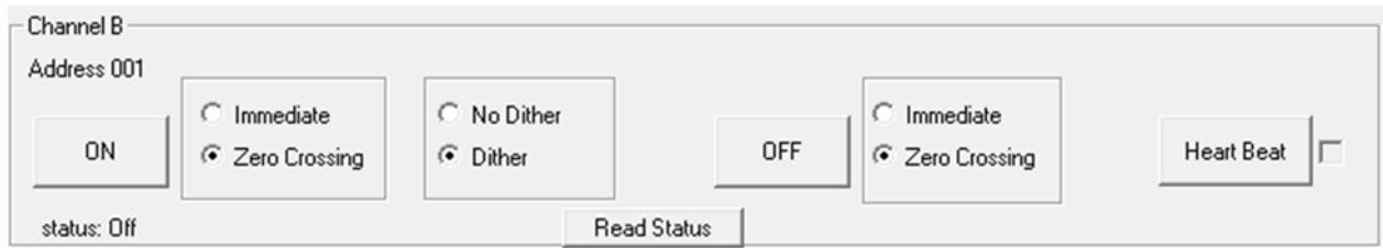
Click the “ON” or “OFF” button to switch on or off the relevant relay (the physical push button on the board are not supported) after selecting the corresponding options.
