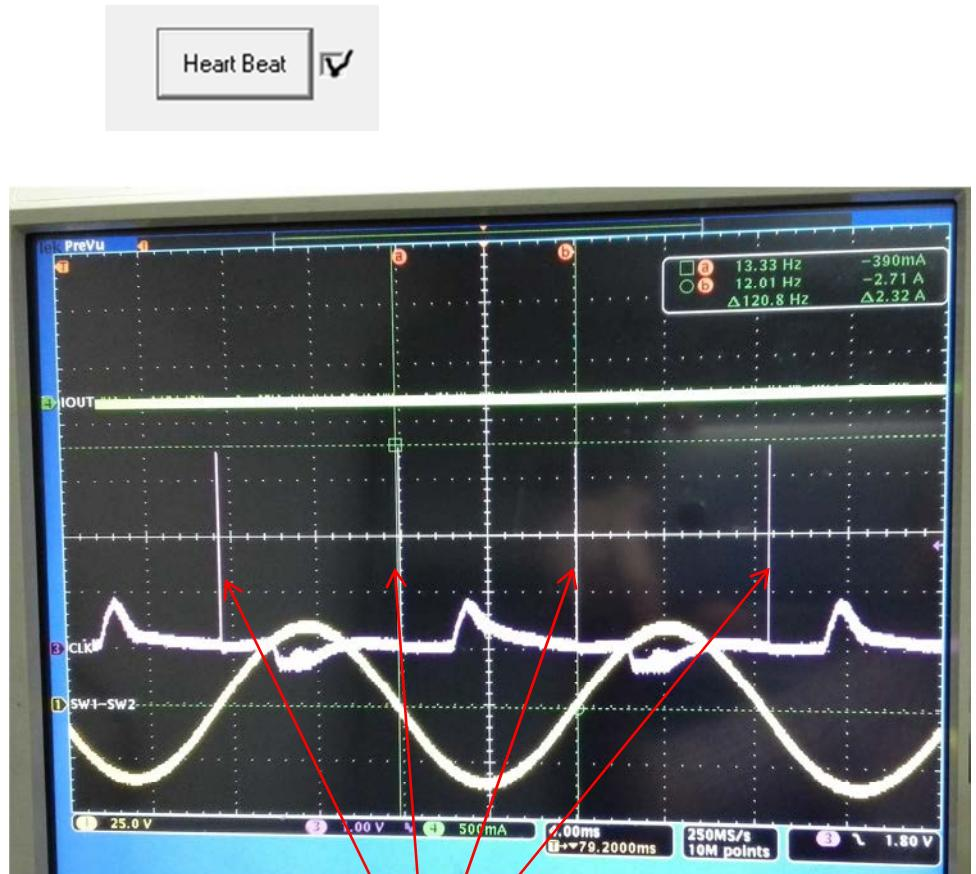
Heart-beat signals sent from DATA pin when the AC waveform is zero crossing.
