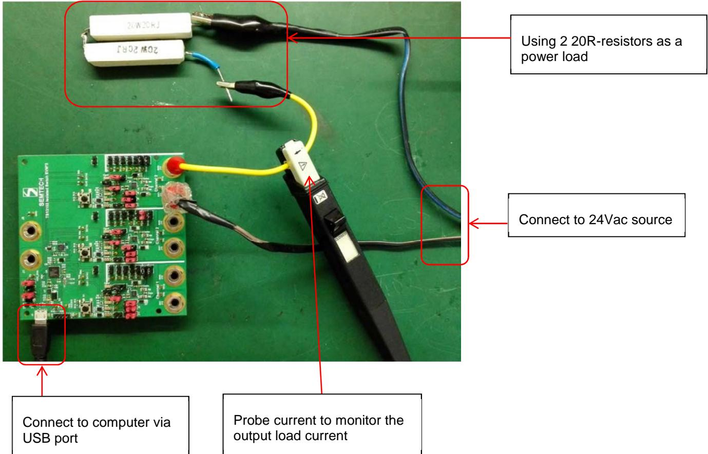
3. Connect the USB cable between TS13102EVM and computer.
