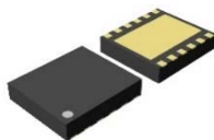
DFN(PLP)2730-12 2.70 x 3.00 x 0.6 (1) mm ( (1) ) maximum dimension
