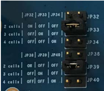
Figure 3-1 JP32/JP33/JP34/JP38/JP39/JP40 jumpers on RTK-251-1PowerBank3.
