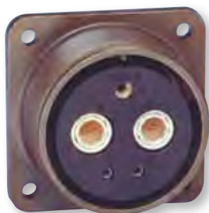
Amphenol 5015 connector with insert pattern 28-5 with (2) size 4 RADSOK® sockets and standard contacts.
