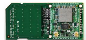
This proven connectivity solution has an SD-card form factor that implements a vendor-independent form factor
