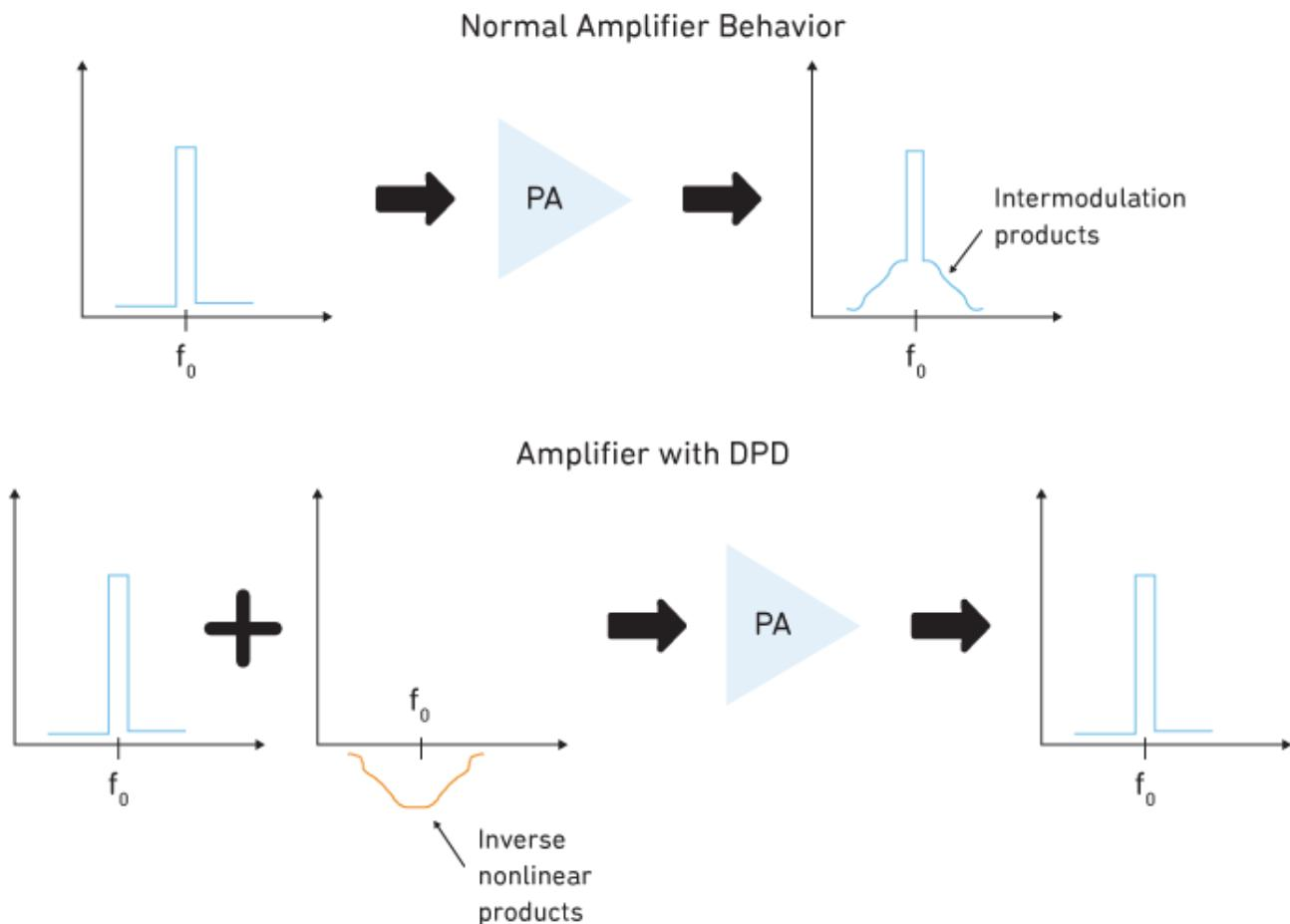
For a CATV optical node, the digital-to-analog converter (DAC) circuit in the node uses software to measure each of the PA outputs through the coupler to determine which PA has the worst linearity. The circuit then calculates a DPD algorithm based on the worst measurement and sends the correction downstream to all the PAs. The worst device is corrected the most, and the end result is multiple devices that run better than without the DPD algorithm.
