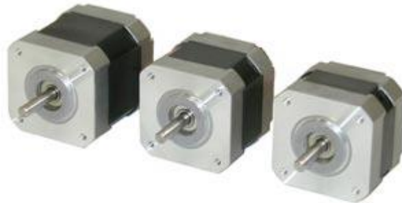
Figure 7: The HT17-268D stepper motor from Applied Motion Products is a representative unit with an industry-standard NEMA 17 frame and mounting holes. Key specifications include 1.8° step angle, 1.34 A/pole current, 31.2 oz-in minimum holding torque and 5.38 oz-in 2 rotor inertia. (Source: Mouser Electronics)
