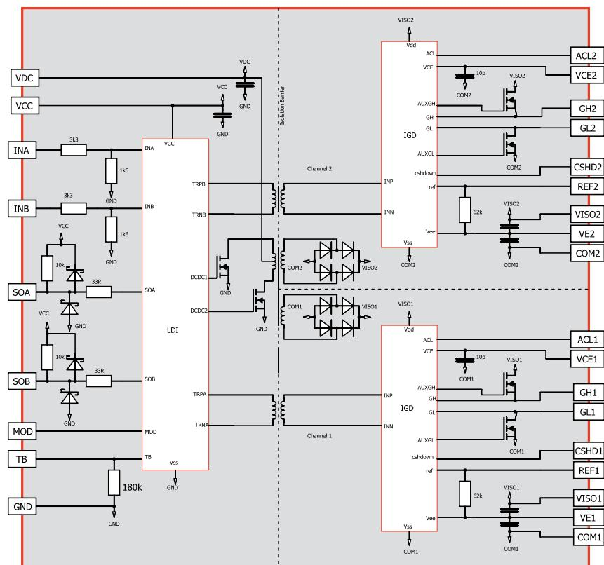
The 2SC0635T2A0-45 combines a complete two channel driver core with all components required for driving, such as an isolated DC/DC converter, short circuit protection, Advanced Active Clamping as well as supply voltage monitoring. Each of the two output channels is electrically isolated from the primary side and from the other secondary channel.
