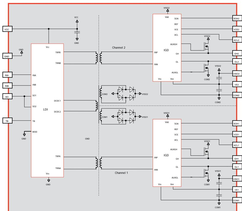
The 2SC0115T is a cost-effective driver core equipped with Power Integrations' latest SCALE™-2+ chipset. The SCALE™-2 chipset consists of two application specific integrated circuits (ASICs) that cover the main range of functions needed to design intelligent gate drivers. It comprises all functionality for an advanced dual channel IGBT gate driver including an isolated DC/DC converter, short circuit protection, Advanced Active Clamping (AAC) and supply voltage monitoring.
