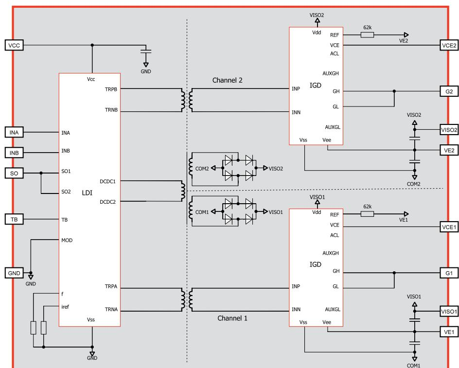
The 2SC0106T is a cost-effective driver core equipped with Power Integrations' latest SCALE™-2+ chipset. The chipset consists of two ASICs that provide the main functions required to implement intelligent gate drivers. Devices include all functionality necessary for an advanced dual channel gate driver: isolated DC/DC converter, short circuit protection, Soft Shut Down (SSD) and supply voltage monitoring.
