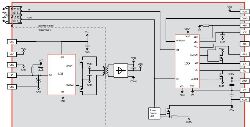
The 1SC0450V2A0-xx combines a complete single channel driver core with all components required for driving, such as an isolated DC/DC converter, short circuit protection, Advanced Active Clamping as well as supply voltage monitoring. Enhanced features such as gate boosting or power supply short circuit protection are also implemented and provide further driving benefits.
