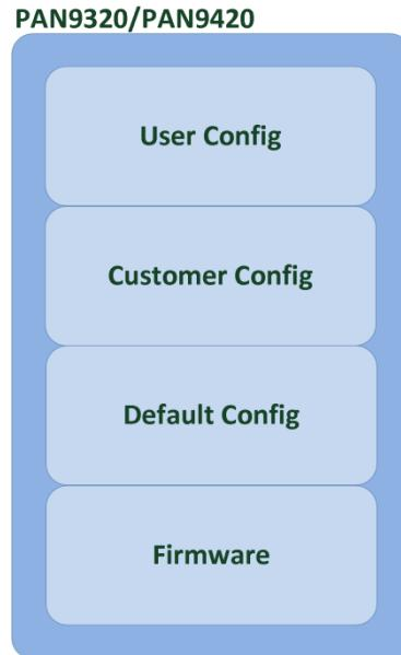
The basis of the PAN9x20 configuration layout is the module firmware with the bootloader and radio driver. The behavior of this firmware can be configured over three configuration layers of which only two can be used by the customer. The default configuration is done by Panasonic in order not to endanger the certification of the module and the end application.
