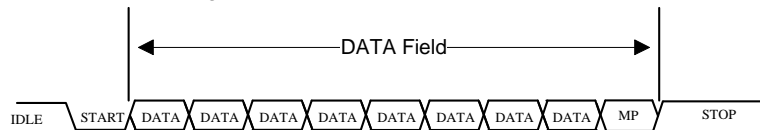
Figure 15-13. UART MP Data Frame
