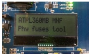
Figure 3-3. LCD Content for PHY Fuses Tool Firmware on PL360MB Evaluation Kit
