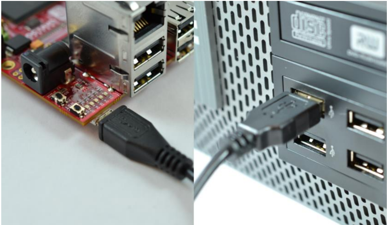
Figure 2: Powering the board using a USB cable
