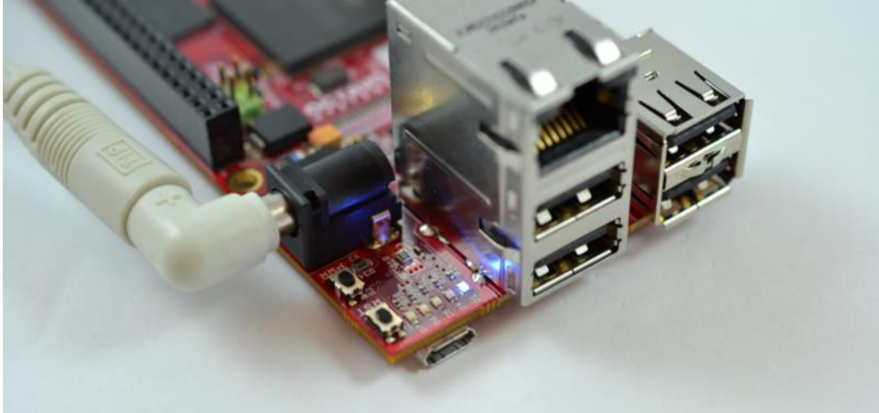
Figure 10: AC-DC adapter plugged in to RED board
