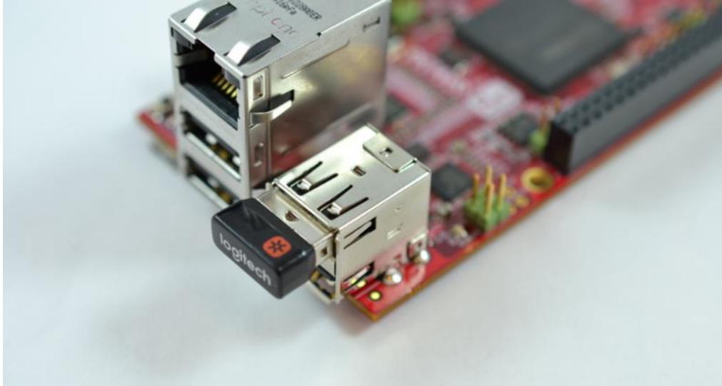
Figure 8: Wireless adapter for keyboard and mouse plugged in to RED board
