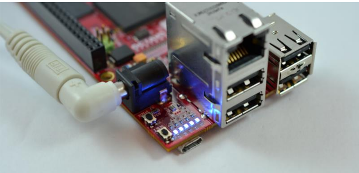
Figure 6: RED board boot up - LEDs D4 - D7 turn ON
