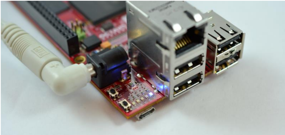
Figure 5: RED board boot up - LED D1 ON
