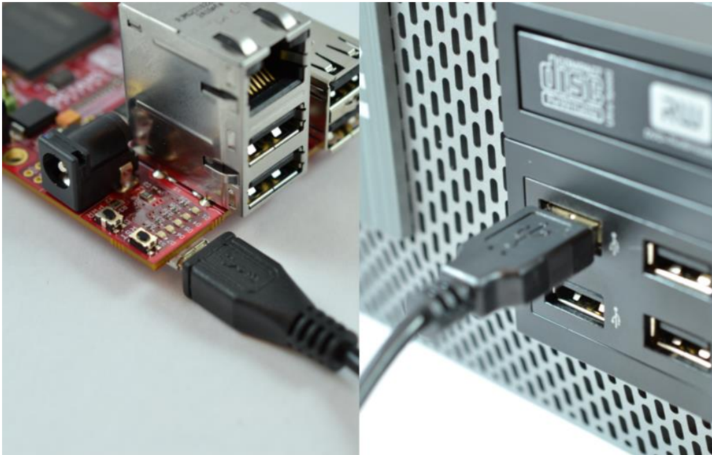
Figure 13: Powering RED board using a USB cable
