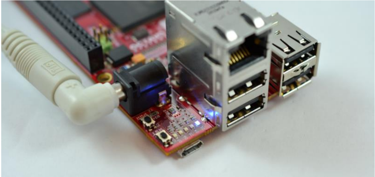
Figure 3: Powering the RED board using an AC-DC adapter
