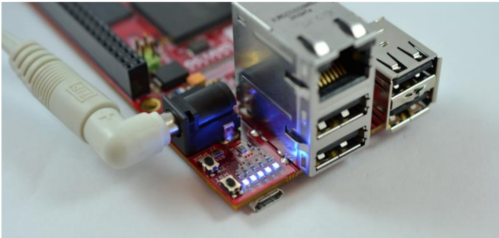
Figure 10: RED board boot up - LEDs D4 - D7 turn ON
