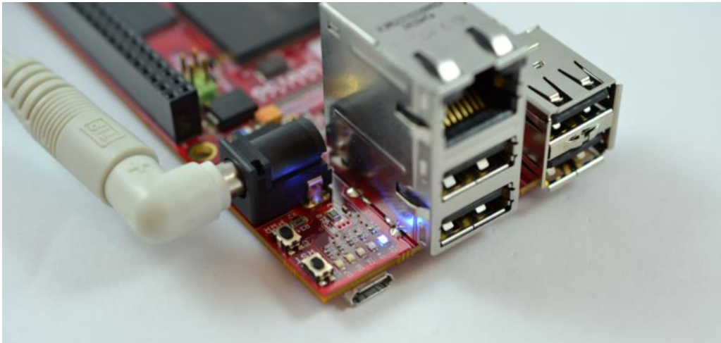
Figure 9: RED board boot up - LED D1 ON
