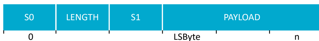
Figure 92: Representation of a RADIO packet in RAM
