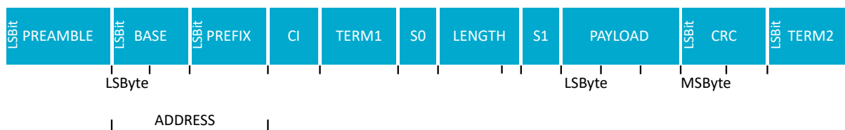
Figure 91: On-air packet layout for Long Range (125 kbps and 500 kbps) Bluetooth Low Energy modes
