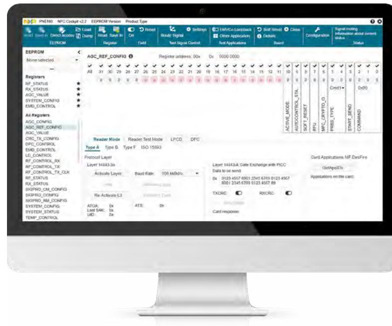
The CLRC663 *plus*, the PN5180, and the PN7462 family are supported by the NFC Cockpit, an intuitive graphical user interface (GUI) that lets you configure and adapt IC settings without writing a single line of software code.
