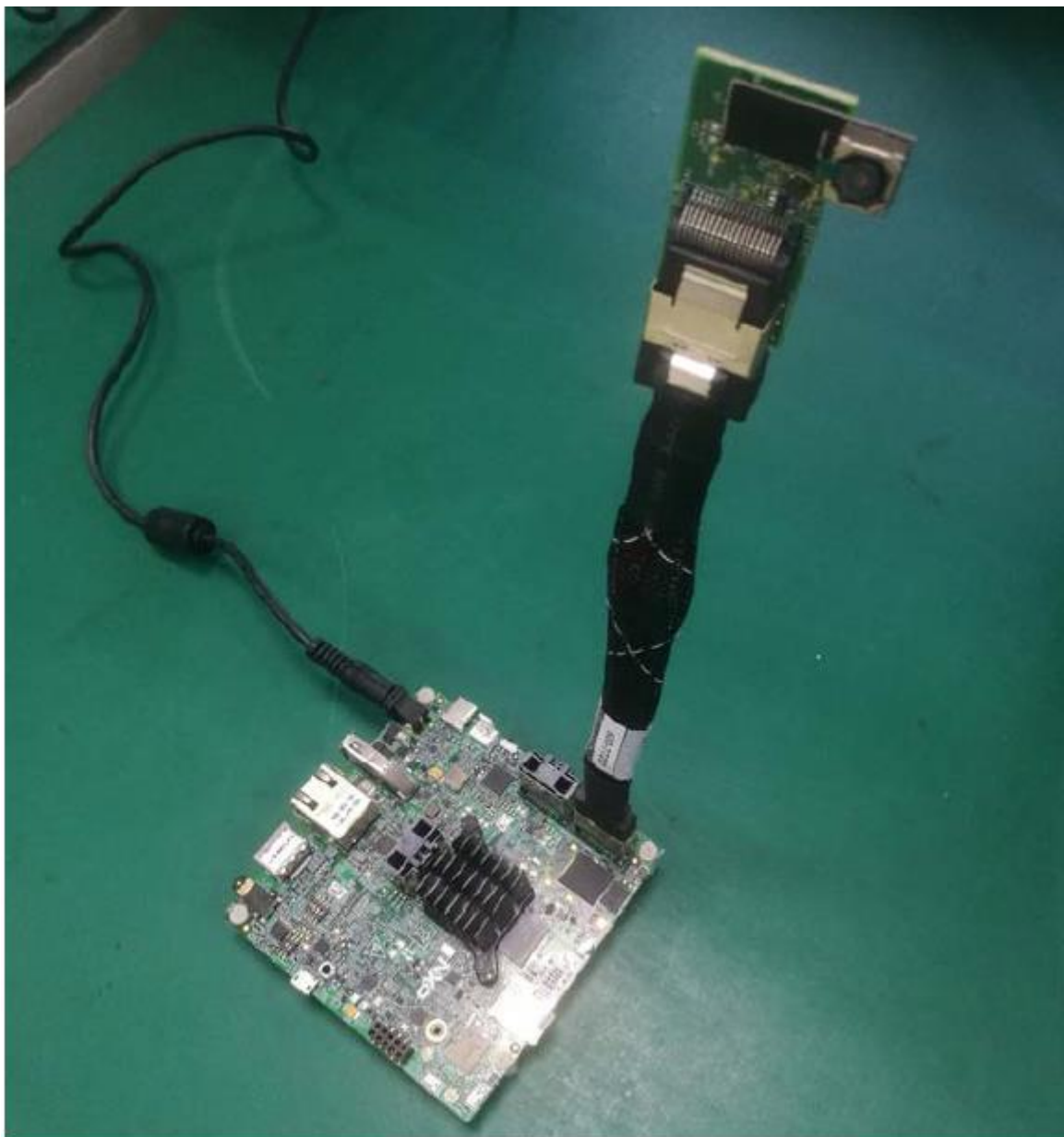
Figure 2. Hardware Setup of MINISASTOCSI Accessory card
