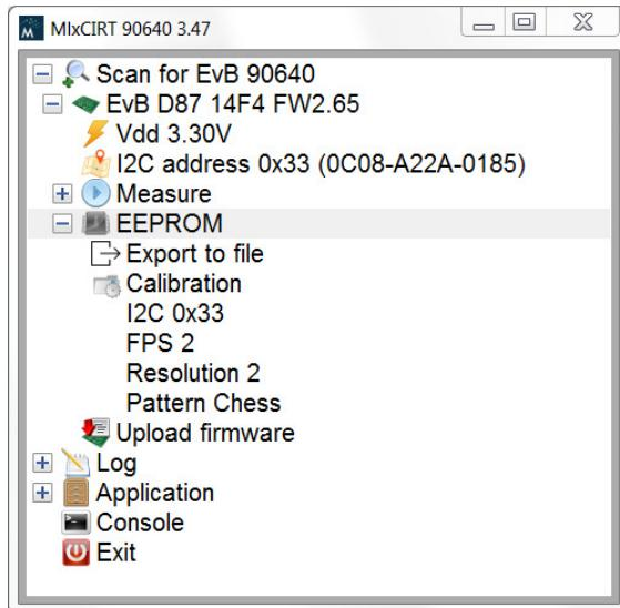
Under the EEPROM tab there is also a tab to export the EEPROM information to file and a button to upload new firmware to the EVB if needed. Here is also a tab to point the program to the file directory where a special calibration file for a specific sensor is located – if available.
