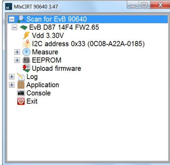
The EVB has been recognized and a sensor has been found on the PCB. The I2C address of the sensor is shown and its factory ID.
