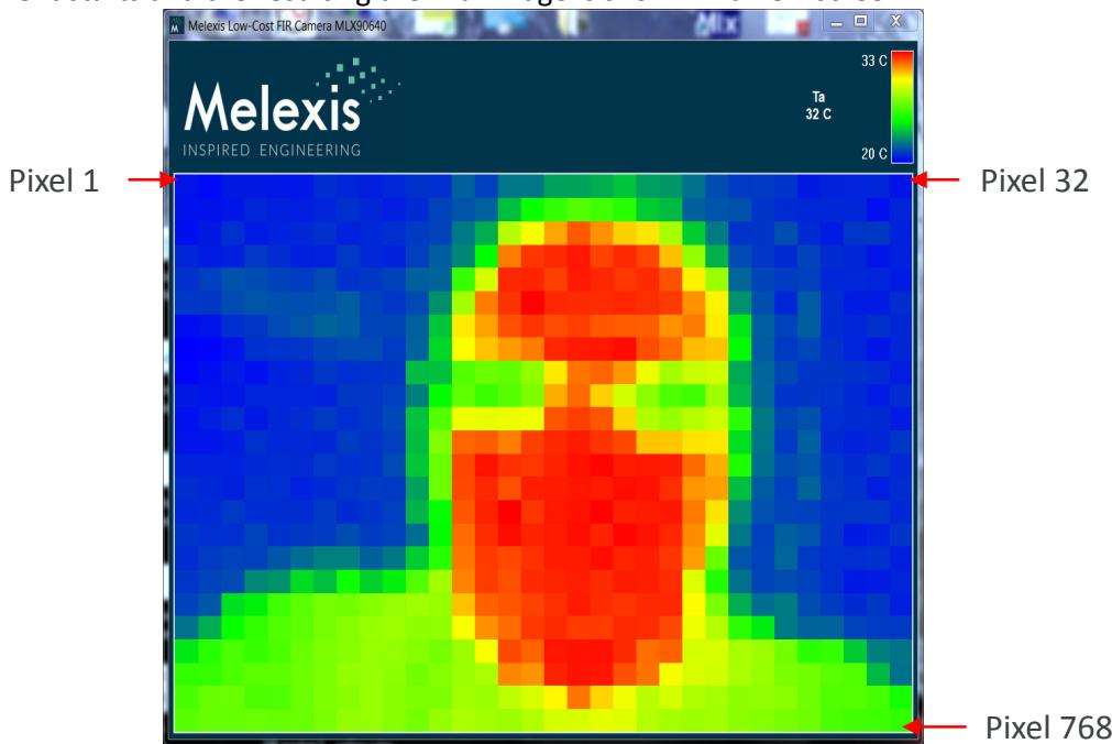
In the top right corner one can see the maximum and minimum temperature of the temperature scale, the sensor temperature  $T_a$  and the temperature  $T_o$  of the pixel at the pointer location.
