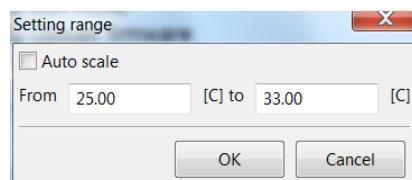
In the “Range” tab one can choose between autoscale or set the minimum and maximum temperature manually.
