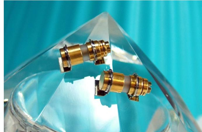
The V9000 Sapphire trimmer capacitor is unique in design. It is truly sub-miniature at just 0.64" (at minimum capacitance) in length, but offers the highest working voltage rating (2 kV) for its size - whilst delivering a capacitance range of 1 to 12pF. Sapphire is ideal for precision trimmer capacitors as its dielectric constant is extremely stable, measuring below 0.0003 up to 10 GHz, and is chemically inert; totally moisture resistant and mechanically strong.
