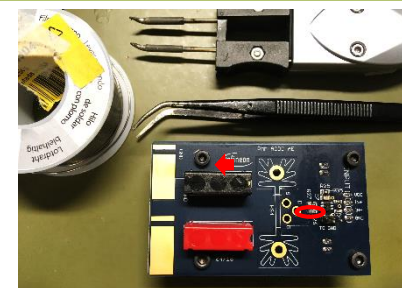
Step 6 Heatsink mounting
