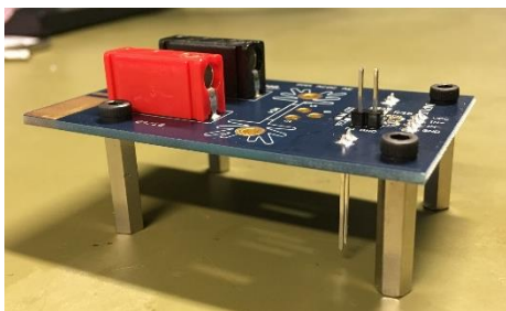
Step 4 TO-220 socket soldering
