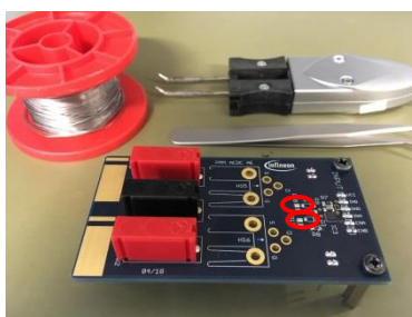
Step 5 MOSFETs placement into the sockets
