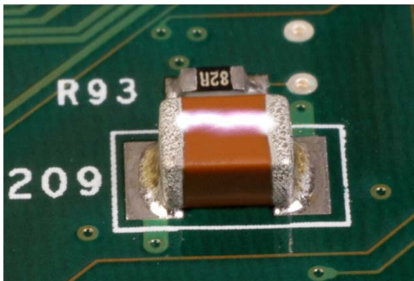
Figure 4. Surface Arcing in an MLCC
