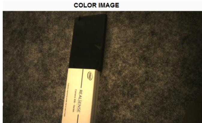
Figure 7. Test scene as seen through the left stereo imager on an Intel RealSense D415 depth camera. This is a RealSense packaging box and a black shiny leather notebook in front of a textured background. Resolution 1280x720. (Note: This is not using the 3 rd color camera in the system).
