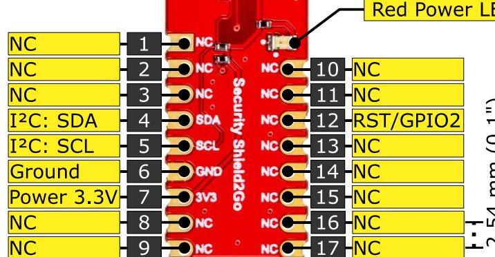
**i** Although labelled as NC, RST is connected to pin 12. This is a mistake of the labelling.
