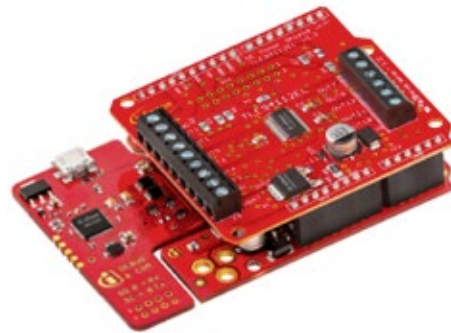
DC motor control with multi half-bridge TLE94112EL
