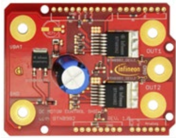
DC motor control with half-bridge BTN8982
