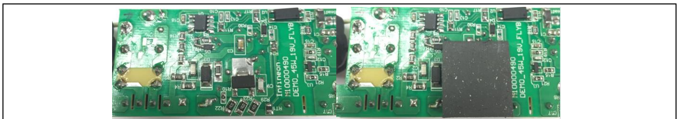
Figure 40 Thermal pad from MOSFET to bottom side
