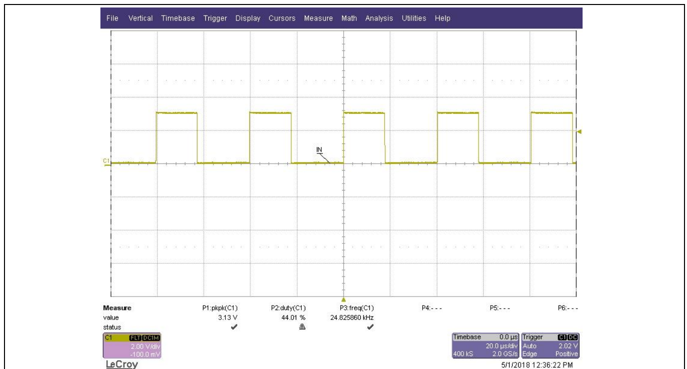
Figure 5 Onboard pulse-signal generator output (C1: IN)
