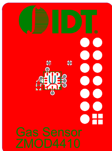
Figure 10. Sensor Board Layout – Top Layer
