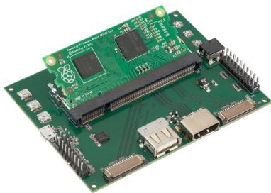
Use the Gumstix Pi Compute FastFlash to upload the latest disk image to your Raspberry Pi Compute Module (not included).
