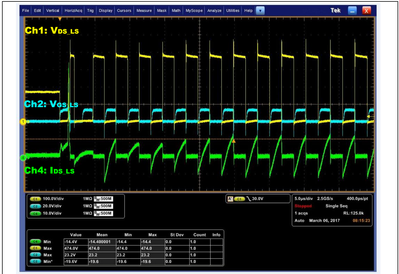
Figure 24 Hard commutation during burst mode operation, V_{DS\_pk} , V_{GS\_max/min} and I_{DS\_MAX}
