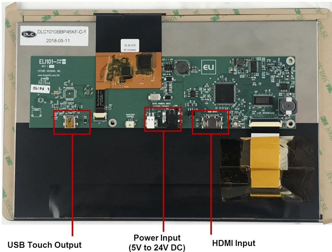
*Power may be supplied either via the 2-pin terminal block J6 or via the 2.1mm power jack P2 (center positive)*
