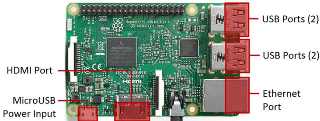
Figure 6. Raspberry Pi 3 Model B Connections
