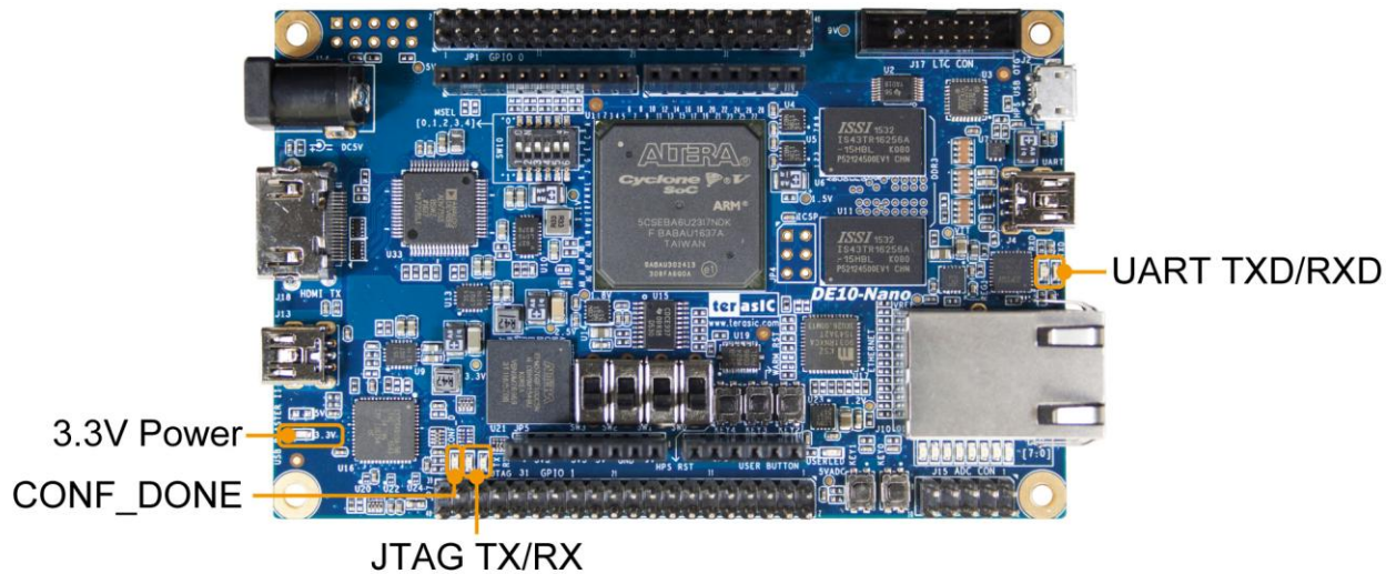
Figure 3-12 LED Indicators on DE10-Nano
